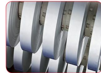
Here you can see an example of applied bonding completed with the help of extensive expertise. A customer requires a liner, which can be easily removed without eating up time. The solution: The fully-surfaced Acrylic-Foam was first furnished with finger lift silicon paper by KMB to allow for easy and clean separating; it was subsequently cut into thin strips.
